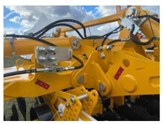
UNFOLDING SYSTEM WITH HYDRAULIC PROTECTION
